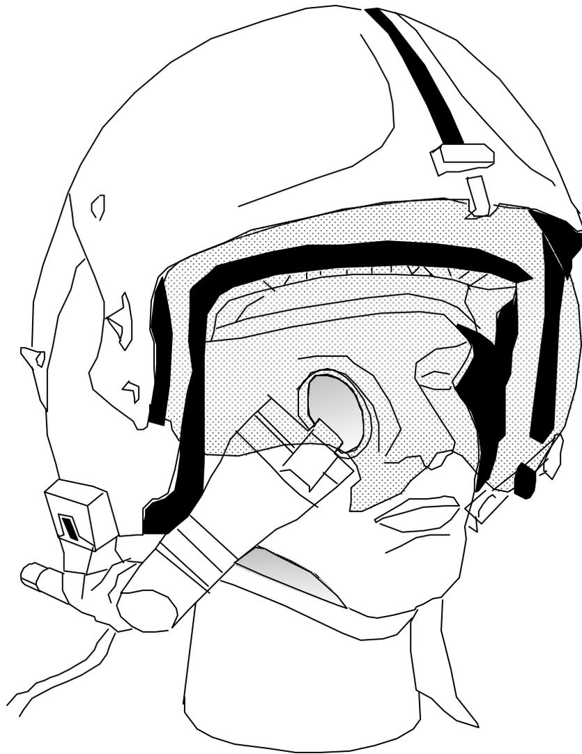
Figure 1. The Integrated Helmet and Display Sighting System (IHADSS) helmet.
